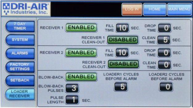
For those dryers with the closed-loop loader option to load the dried material to the press, this screen is used to configure the loading cycle.
