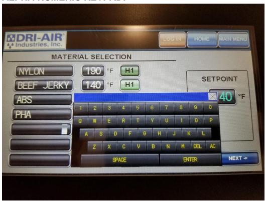
To enter a new recipe or other designation, press the center description area and the keypad as shown will appear. Type the new entry using the keypad and press enter.
