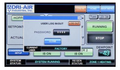
In addition, switching between Fahrenheit and Celsius can only be done under factory settings.
